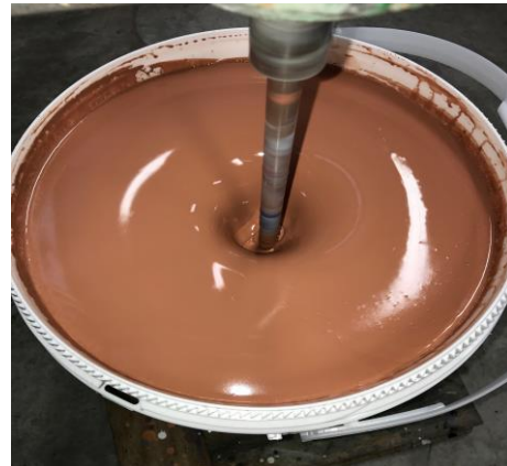
Use a slow mixer (200-300rpm) and create a vortex without drawing air into the coating.
