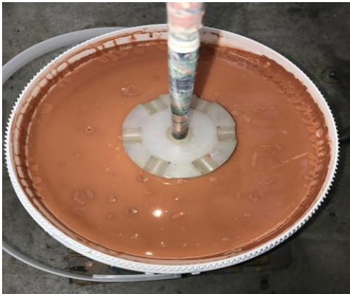
Use a mixing disc with a diameter of approximately 1/3 rd the diameter of the pail.
