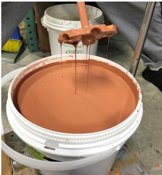
Coating is properly mixed when removing the mixing disc from the pail, the coating flows smoothly like oil without dripping.
