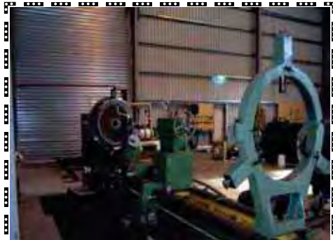
No. CW62143C CENTRE LATHE 1480mm swing over bed and 4.5m between
